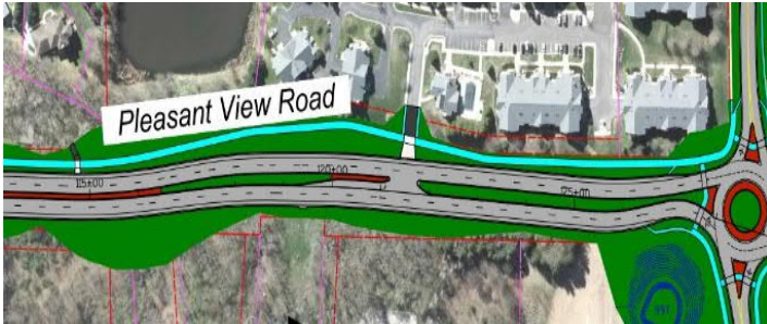
Pleasant View Road is a high traffic volume corridor currently without pedestrian/bike accommodations. The graphic above shows proposed sidewalk/path (in blue) on one side only to limit property impacts potentially similar to the Libal Street project.
