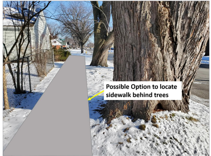
Potential option for location of sidewalk behind large and mature trees to avoid impacting the trees.
